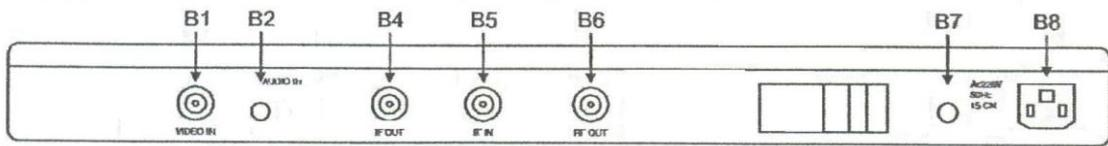
B1 Video input port (VIDEO IN) input Video Signal 1Vp-p, input impedance  $75\Omega$
